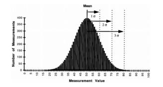
Fig. 7. Frequency distribution according to Gauss of measured values centered around an average value
