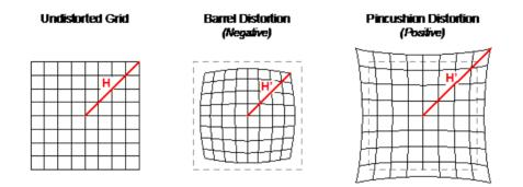
Fig. 6. Local geometric distortions caused by optical imaging (lense distortion)
