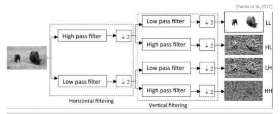
Fig. 3. Decomposition of an image 2-D discrete wavelet transform with filter banks (2-D DWT)
