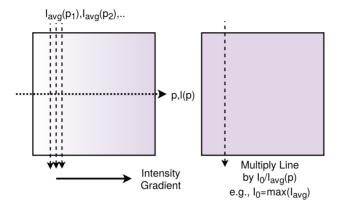
Fig. 2. (Left) Computing the average intensity  $I_{avg}(p)$  perpendicular to a line along the intensity gradient (Right) Correct all pixels perpendicular to the correction line with a equalization factor
