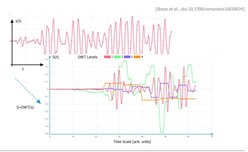
Fig. 4. Example of a DWT signal decomposition of a US time-dependent signal
